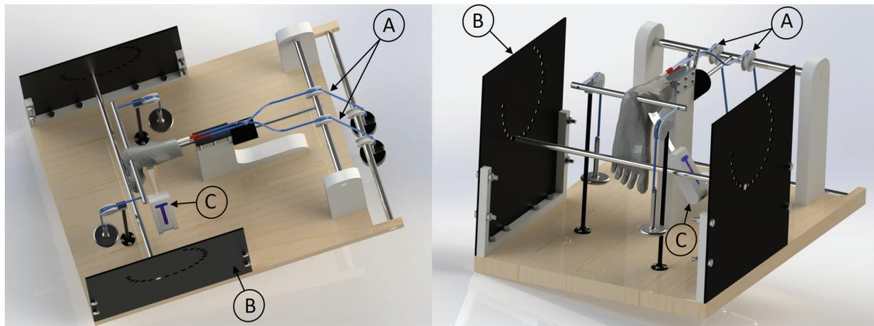
**Figure 1.** The ankle test rig: muscle loading system (A), a slot-and-bar system (B) to allow the ankle to be dorsiflexed and plantarflexed and to enable it to be held in a standardized position for testing, and Tekscan film and handle (C).
