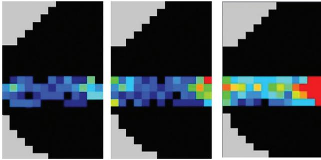
**Figure 2.** Screen Tekscan image of the pressure reading from 1 ankle: on the left, in plantargrade and neutral hindfoot alignment; in the center, in full plantarflexion and neutral alignment; on the right, in full plantarflexion with valgus hindfoot alignment. Pressures rise during plantarflexion and then further with valgus combined. This was a typical pattern observed for most ankles. Scale: dark blue, close to zero pressure; midgreen, 0.4 MPa; red, 0.6 MPa.
